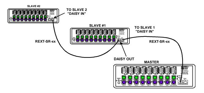
Figure 7- Connect remote extension cables between cascaded units
